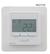
Multireg LCD2 is an electronic thermostat with four functions. Room sensor, floor sensor, power regulator and maximum / minimum limiter. The thermostat has a backlit LCD-display and weekly programming.
