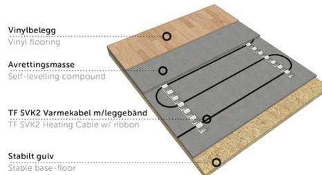
**TF SVK2 17W Heating Cable can be ordered from [thermo-floor.no](http://thermo-floor.no)**
