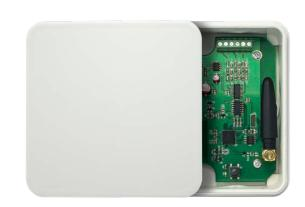
Heatit Z-Relay multipurpose relay module may be used for many different applications. The IP 55 rated casing makes it useful for any outdoor application. Can pull loads up to 25A.
