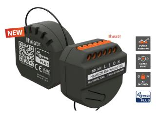
Heatit ZM Thermostat is an electronic thermostat for electrical underfloor heating designed for inwall installations. The thermostat allows you to control your electrical heating through your Z-Wave network. The module is equipped with a 16A single pole relay. The thermostat requires you to connect an external wired sensor which is included with the device. The device can withstand a max load of 16A at 230VAC.
